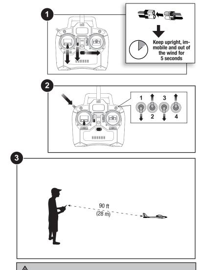
**CAUTION:** While holding the aircraft during the Range Test, always keep body parts and loose items away from the propeller. Failure to do so could cause personal injury.
